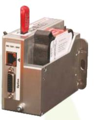
USB stick data transfer Dynamicaly transfers Data created with a PC to the printer
